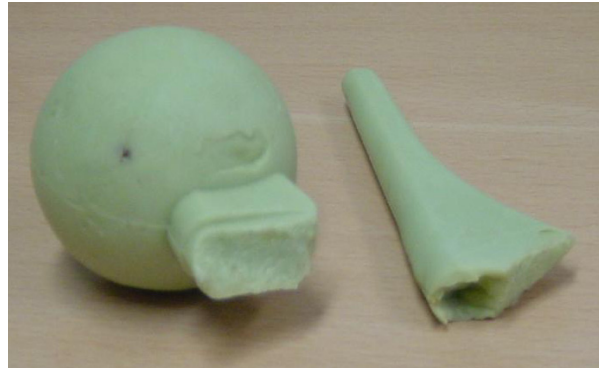
Figure 3. The fractured cement spacer mould as removed from the hip.
